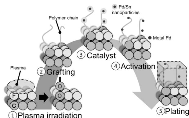
Fig. 1 Surface metallization process of PTFE
