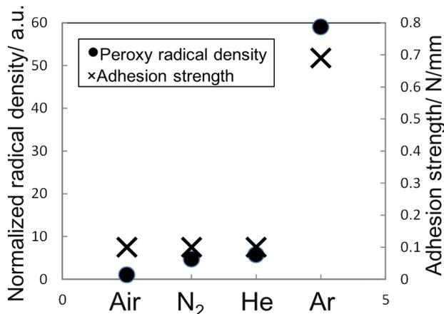
Fig. 4 Effect of gas type on peroxy radical density and adhesion strength of Cu layer on PTFE. Each plasma irradiation time was 20 min.
