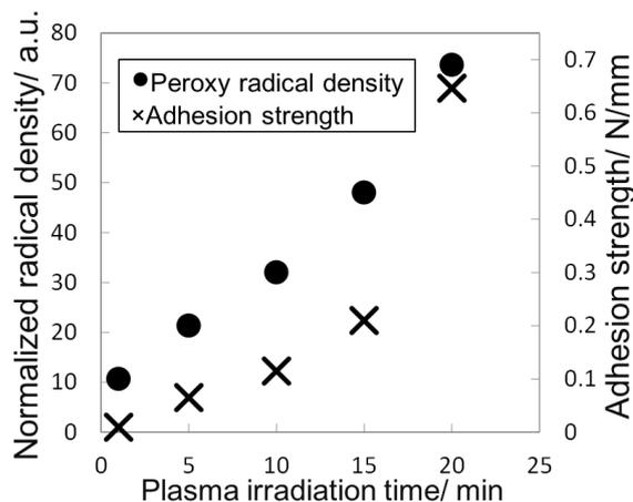
Fig. 5 Effect of Ar plasma treatment time on peroxy radical density and adhesion strength of Cu layer on PTFE.
