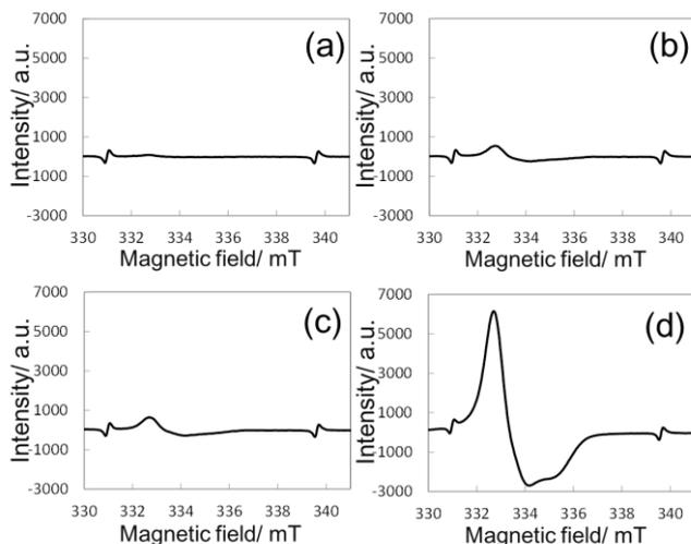
Fig. 3 ESR spectra of PTFE surface irradiated with four kinds of plasma at atmospheric pressure. (a) air, (b) N<sub>2</sub>, (c) He, (d) Ar. Each plasma irradiation time was 20 min.
