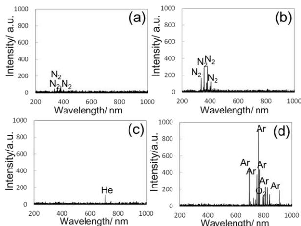
Fig. 2 Optical emission spectra of four kinds of plasma at atmospheric pressure. (a) air, (b) N<sub>2</sub>, (c) He, (d) Ar.
